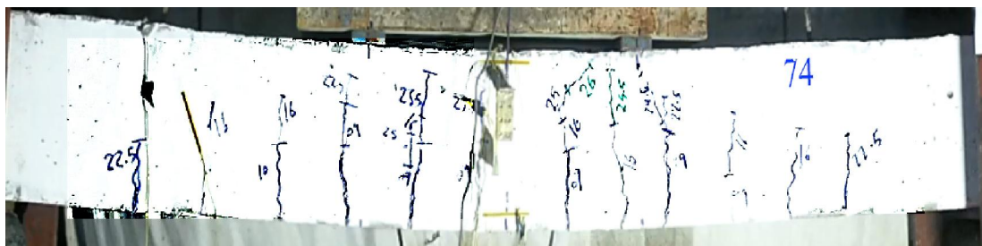
Figure 7: Crack pattern of the control sample 74.
